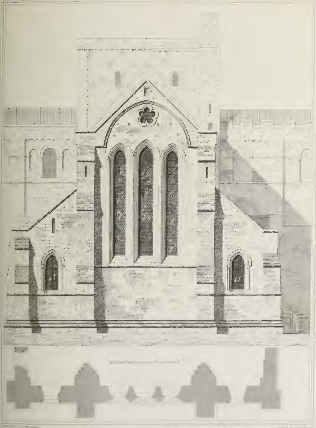
Elevation of the window in the choir of the church of St. John the Baptist, Bath, Somerset, England. The window is of the 13th century. The plan shows the window in its position in the choir.
